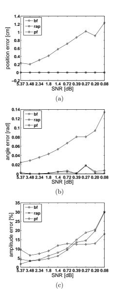
FIGURE 1. Low signal-to-noise ratio: reconstruction error for the position (a), orientation (b) and amplitude (c) of the three algorithms in the case of the data with different signal-to-noise ratio.
