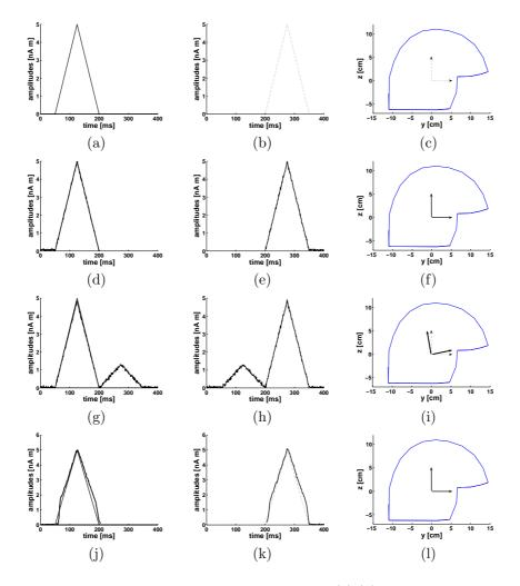
FIGURE 2. Orthogonal dipoles: amplitudes (a),(b) and projection on the sagittal plane (c) of the original dipoles; reconstructed amplitudes (d),(e) and projections (f), obtained with the beamformer, with RAP-MUSIC (shown in (g),(h) and (i)) and with the particle filter (shown in (j),(k) and (l)).
